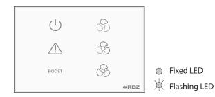
**NO COMMUNICATION** - When the LEDs light up in succession with a circular effect and with a duration of more than 60 seconds, this indicates a failure of communication with the bus network.
